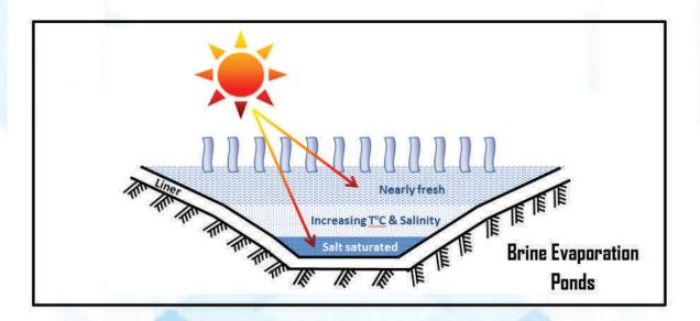
Brine is allowed to evaporate in ponds while the remaining salts accumulate in the base of the pond
